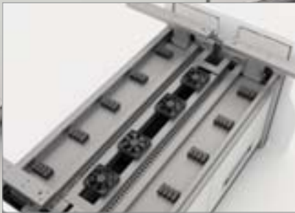
Fan installed to boost the natural convection.
